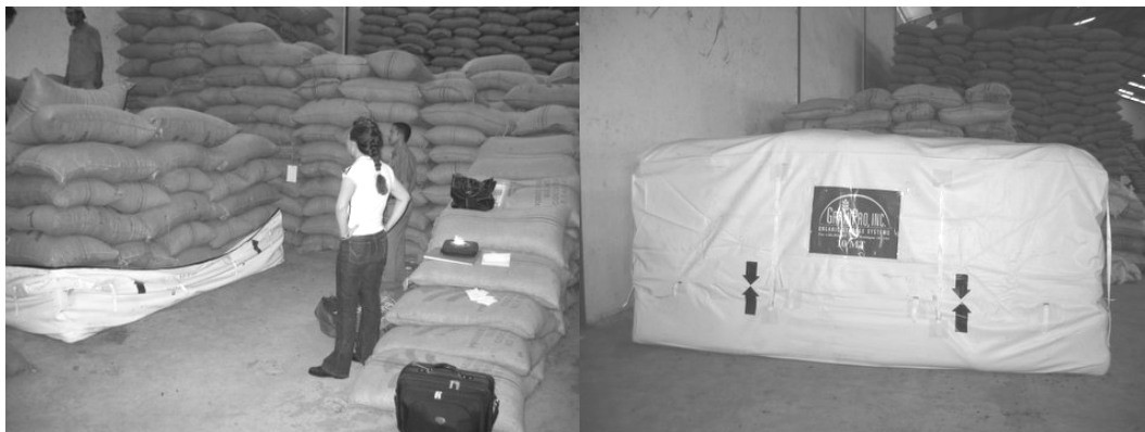
Fig. 5. The GrainPro cocoon, before sealing (left) and after sealing (right) (courtesy of Tom deBruin).
